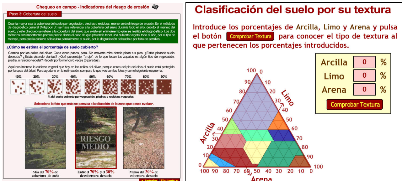
Figure 3. Screen shots of interactive graphs for evaluating the erosion risk using field indicators (left) and for providing the soil texture class from particle-size distribution data.
