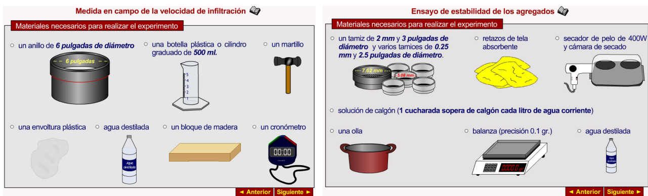
Figure 2. Screen shots of the required materials to execute simple field experiments. Measurement of infiltration rate (left) and aggregate stability (right).
